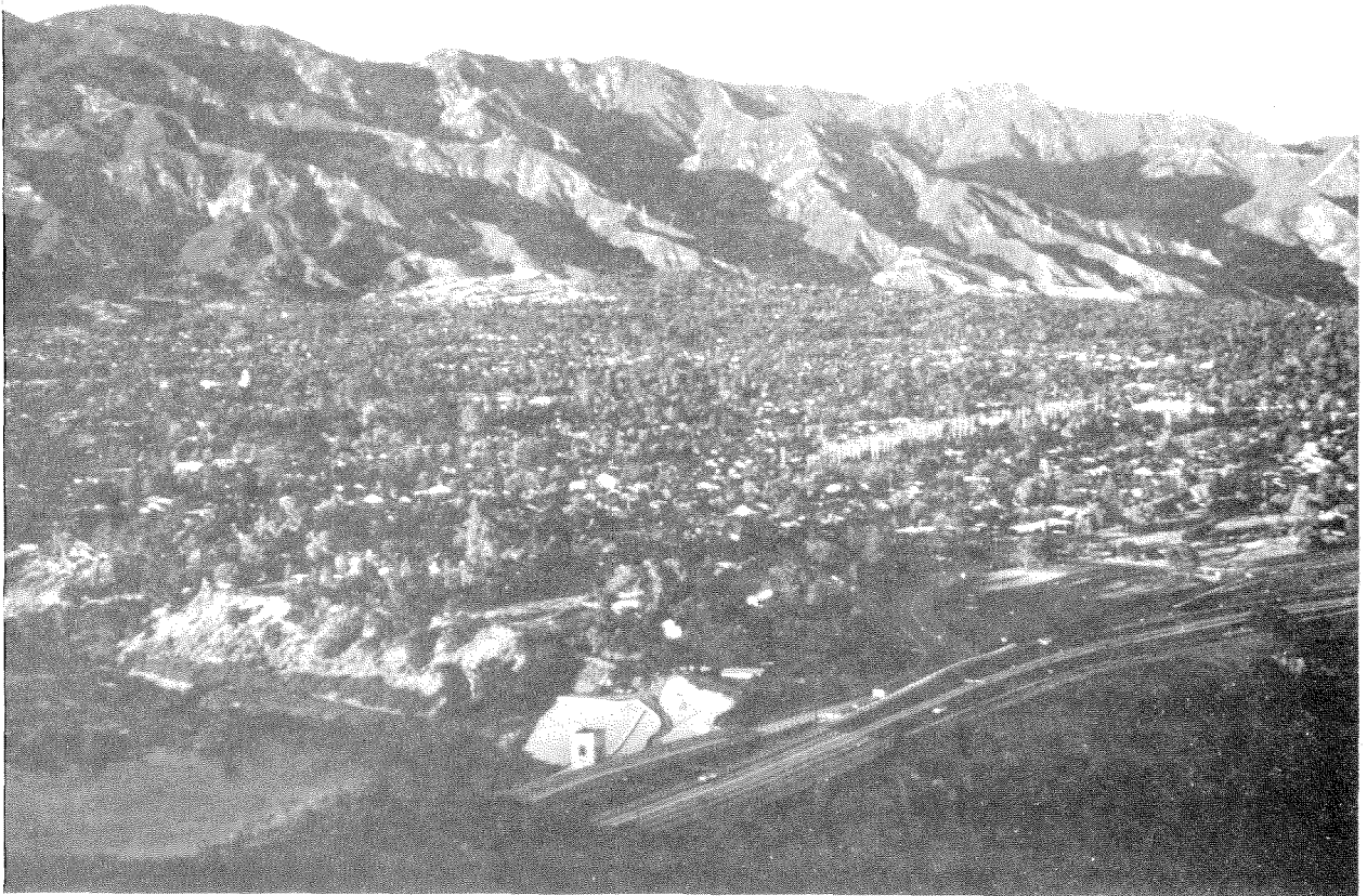
FIGURE 3 The San Gabriel Mountains drain from steep canyons directly onto alluvial fans, such as this large one underlying Altadena and the northern part of Pasadena (northeast of Los Angeles). The developed areas on this fan are protected by debris basins at the mouths of the canyons (see Figure 4).
